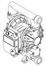
The GRACO QUANTM<sup>™</sup> electric operated diapragm pump combine all of the benefits of a traditional air operated diaphragm pump like self-priming, stalling under pressure and increased diaphragm life with the benefits of an electric pump like energy cost savings, reduced pulsation and increased pump control.
