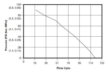
Performance may vary based on pump materials, suction condition, discharge pressure, and fluid type.
